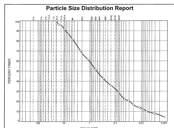
GRAIN SIZE - mm. % Fines % Gravel % Sand % Cobbles Coarse Medium Fine Silt Clay Fine Coarse 0 22.3 6.5 0.0 0.0 18.1 14.2 20.8 18.1
