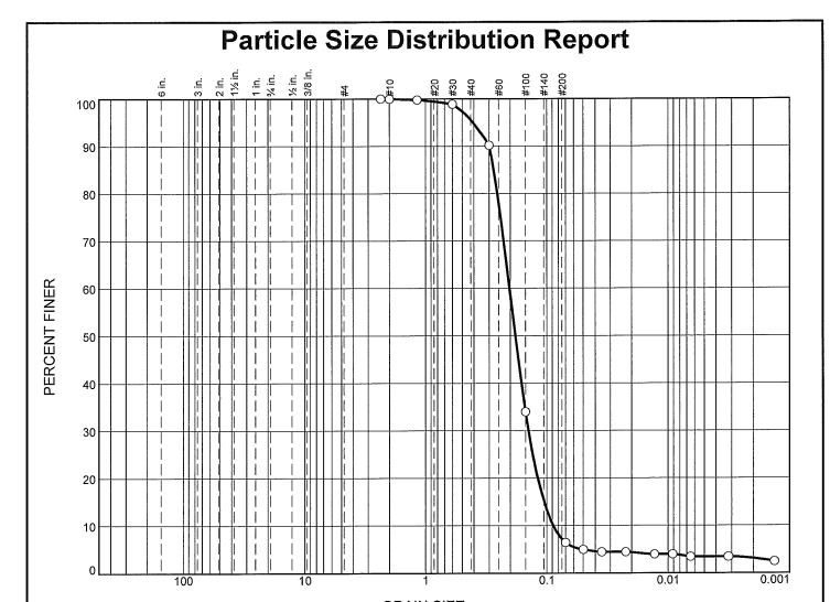
GRAIN SIZE - mm. % Fines % Gravel % Sand % Cobbles Clay Medium Fine Silt Coarse Fine Coarse 88.3 4.1 3.1 0 0.0 0.0 0.0 0.0 4.5
