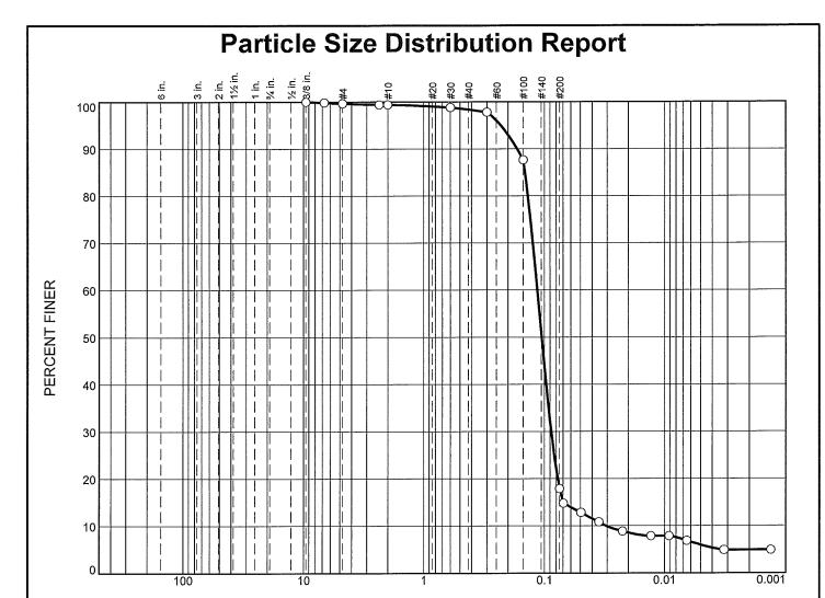
GRAIN SIZE - mm. % Fines % Gravel % Sand % Cobbles Fine Silt Clay Coarse Fine Coarse Medium 0 0.0 80.5 13.0 4.9 0.0 0.3 0.3 1.0
