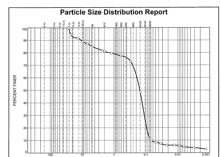
GRAIN SIZE - mm. % Fines % Gravel % Sand % Cobbles Medium Fine Silt Clay Coarse Fine Coarse 0 0.0 7.5 7.6 4.7 65.3 7.7 3.4 3.8
