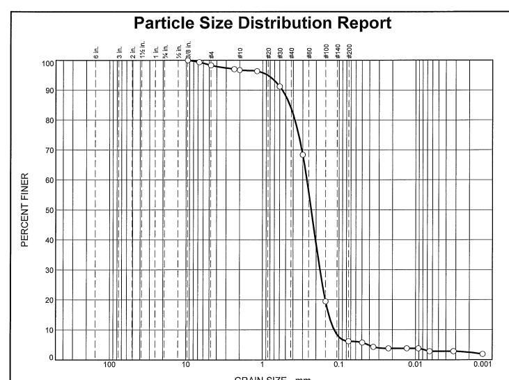
GRAIN SIZE - mm. % Gravel % Fines % Sand % Cobbles Coarse Fine Medium Fine Silt Clay Coarse 0 0.0 0.0 1.7 1.6 12.8 77.7 3.7 2.5
