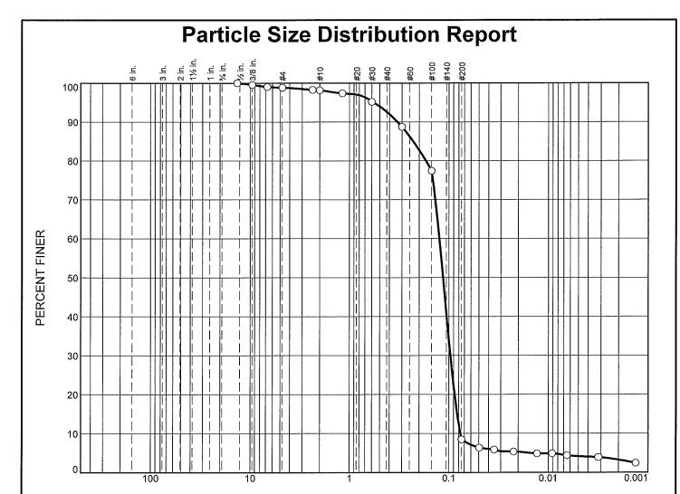
GRAIN SIZE - mm. % Gravel % Sand % Fines % Cobbles Fine Silt Clay Coarse Fine Coarse Medium 0.0 84.2 0.0 1.1 0.7 5.6 5.2 3.2
