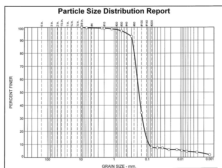
% Fines % Gravel % Sand % Cobbles Silt Clay Coarse Fine Coarse Medium Fine 4.7 0 0.0 0.0 0.5 0.3 3.7 87.8 3.0
