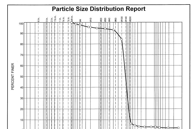
GRAIN SIZE - mm. % Fines % Gravel % Sand % Cobbles Silt Clay Coarse Fine Coarse Medium Fine 0 82.9 2.3 0.0 0.0 2.4 2.1 1.9 8.4
