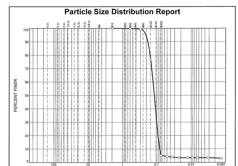
GRAIN SIZE - mm. % Fines % Gravel % Sand % Cobbles Silt Clay Coarse Fine Coarse Medium Fine 0 0.0 94.5 2.0 3.2 0.0 0.0 0.0 0.3
