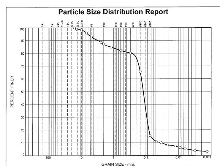
% Fines % Gravel % Sand % Cobbles Clay Coarse Medium Fine Silt Coarse Fine 0 0.0 65.5 12.3 3.3 0.0 7.2 5.6 6.1
