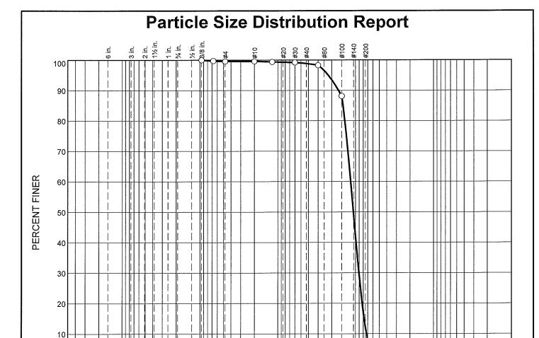
GRAIN SIZE - mm. % Fines % Gravel % Sand % Cobbles Fine Silt Clay Coarse Fine Coarse Medium 0 0.0 87.0 9.4 2.4 0.0 0.4 0.0 0.8
