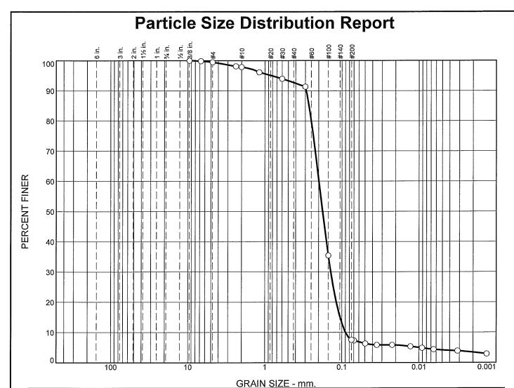
% Gravel % Fines % Sand % Cobbles Clay Coarse Fine Medium Fine Silt Coarse 0 0.0 0.0 0.5 1.6 5.2 85.2 4.1 3.4
